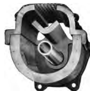
Fig. 4. Section through Wired-Glass Guard.
